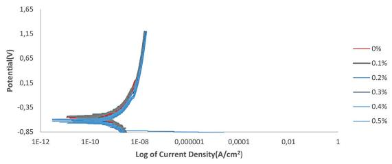
**Fig. 2.** Polarization curves for DSS2101 immersed in 0.5M H<sub>2</sub>SO<sub>4</sub> in the presence and absence of *Hura crepitans* seed extract as inhibitor at 298 K
