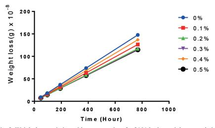
Fig. 3. Weight loss variation with exposure time for 2101duplex stainless sample immersed in 0.5M H<sub>2</sub>SO<sub>4</sub> with various *Hura crepitans* seed extract concentrations
